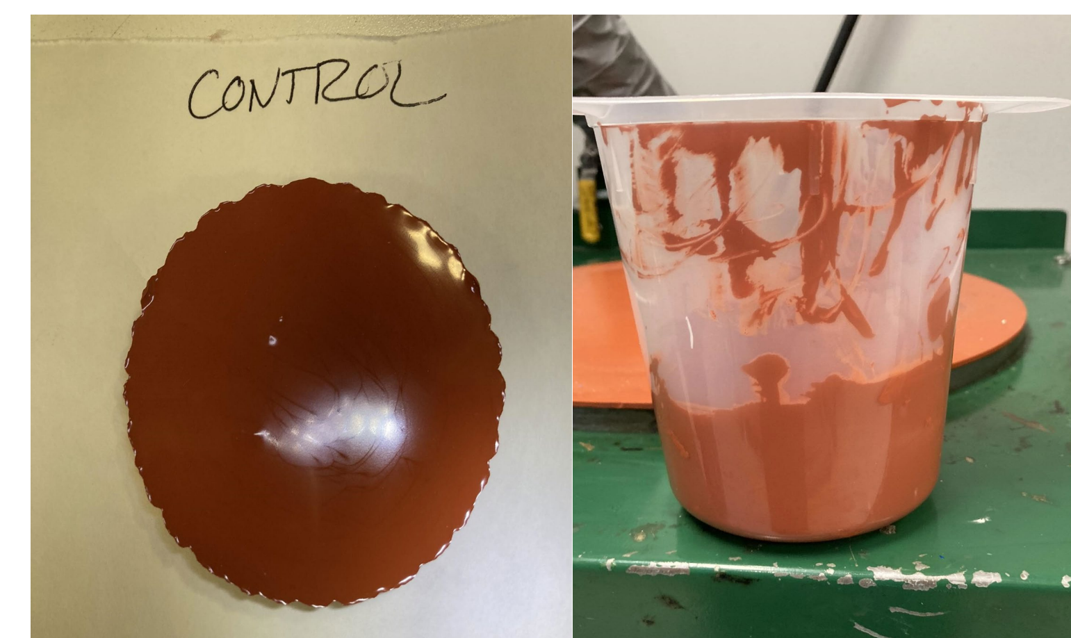
Figure 3. Silicone Puck that was put through testing (left) and the silicone before being mixed (right)
